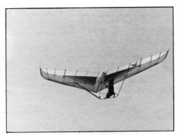
In looking at the above wings, little similarity is obvious, yet more is present than initially meets the eye. Both craft use "wing spars" to bear in-flight loads. The primary difference, and the one causing Hiway to employ the rudders you see, relates to the positioning of the wing spar. By having it forward of the center of lift line at the tip, Pro Air's Dawn retains weight shift control simplicity.
