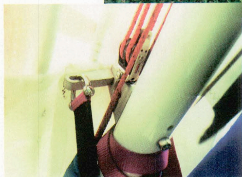
The spreader tower hang mechanism.
