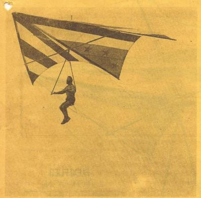
Hang Glider Shoppe now offers the complete planset to the FLEXLELIER. This is a standard Rogallo hang glider; easy to transport, fast to set up and safe to learn on.
