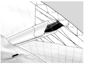
To open or close the batten tip lever press firmly on the undersurface of the tip lever to disengage or engage it (Fig. 10).
