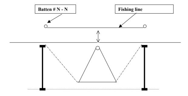
4. Press firmly on the end of each sprog supported batten and then release. Set the VG to full off and than to full tight again. Measure the crossbar travel: it should be 130mm. Measure the height of each thread relative to the top of the keel tube. The results should be as follows:
