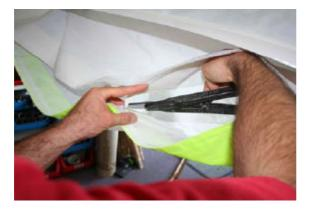
Before moving to the keel, ensure that the outer wing tube is inserted completely into the spar. Look through the hole in the sail.
