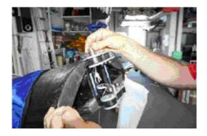
4.) Take the outer wing tube out of the D-spar.
