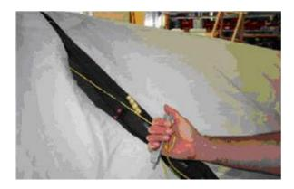
13.) Attach the sail to the keel. Insert the ring and tighten the lever to the opposite side till the spring pin snaps and secures the lever.
