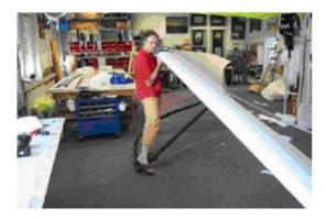
21.) Fix the nose cover. The Velcro has to be replaced if it loses strength. Don't fly with lose nose cover!
