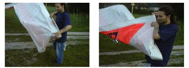
• Holding the extremity of the wing in this position, take the sail by the trailing edge and lift it upwards until it is tight and from this position roll in the sail, starting from the trailing edge.
