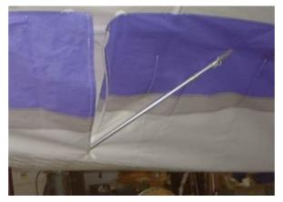
• Open the wingtip zipper and take out the transversal carbon batten.
