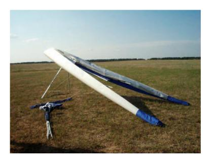
2.2.3. Install the small mast on the LE-tubes/X-beam junction to it's proper place. Dive sticks must be outside of the sail. (Fig. 5).
