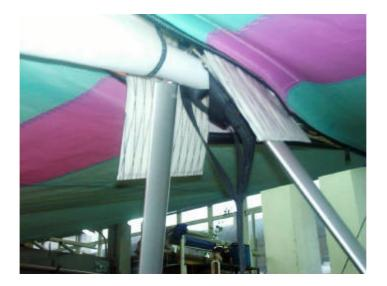
4.1.6. Pull in the wings slightly and remove all battens except the top battens No.1. Remove only the batten spring ends from the trailing edge pockets. Put the battens into the bag. **Do not forget to remove the undersurface battens from the sail !**
