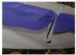
Ø Open the central zipper which is under the keel and check that the T junction, to which the hang strap is attached to, is rotated in perpendicular position to the keel; then close the zipper.
