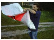
Keeping the end part of the wing in this position, take the sail by the trailing edge and lift it upwards until it is tight and from this position roll up the sail starting from the trailing edge.
