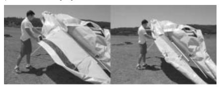
9. Attach ties loosely around glider, going from wing tip to nose, and then tighten the ties, moving from nose to wing tip, adjusting the sail so that the leading edge Mylar inserts overlap smoothly with no kinks, as shown.
