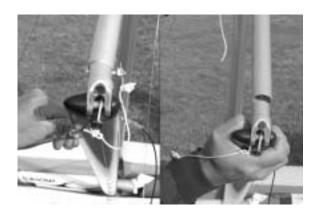
3. Roll the glider over so that it is standing on the control frame.
