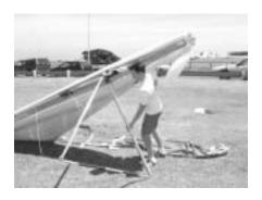
4. Insert the ring of the lower front wires in the Bailey Block making sure that the spring is firmly locked and the wires untwisted.
