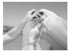
5. Insert the nose batten. The batten may need some "feeding" through the Sail by pulling the sail forward to remove any wrinkles as the batten slides into its pocket.
