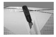
14. Locate the inner and outer wire braced dive struts by placing them inside the sail, below the webbing loop. Note that the action of closing the cord-wise zipper creates the loop necessary to hold the strut in place.
