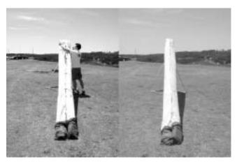
10. Put the glider bag over the glider, and then lay the glider over on its side.
