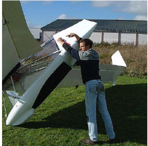
2. With the **left hand** pulling the strap, lift the tail of the Swift up with the right triplet pivoting on the ground.
