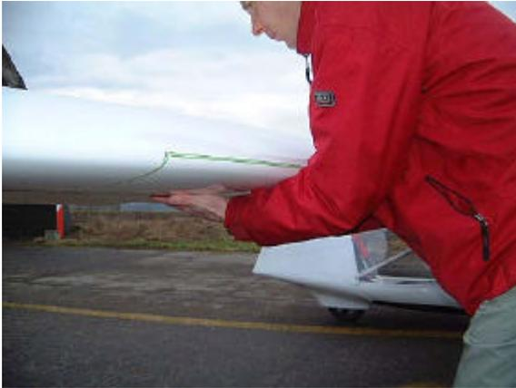
**Always support the wing with flat hands, on the bottom surface and on the spar (the spar is in the thickest part of the airfoil) or at the wing tips.**
