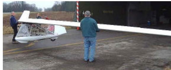
3. With 2 people, each one can carry it a bit further than the level of the vortillons with flat hands. Support and carry the wing at the wing spar (the thickest part of the wing). If the wing pitches back then go further out towards the tip until a balance point is reached.
