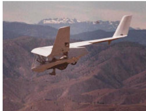
When the pilot is flying in a standing position, the CG position is aft. That is why during T.O. and until the pilot is supine one must keep a bit of forward pressure on the control stick. This peculiarity is a great help during the take off because the elevons facing down together with the flaps increases the lift produce by the wing.
