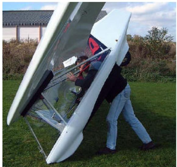
4. Release the lifting handle, which should automatically retract. Put your head, shoulders and left arm inside the trap doors. Put the shoulder straps over your shoulders.
