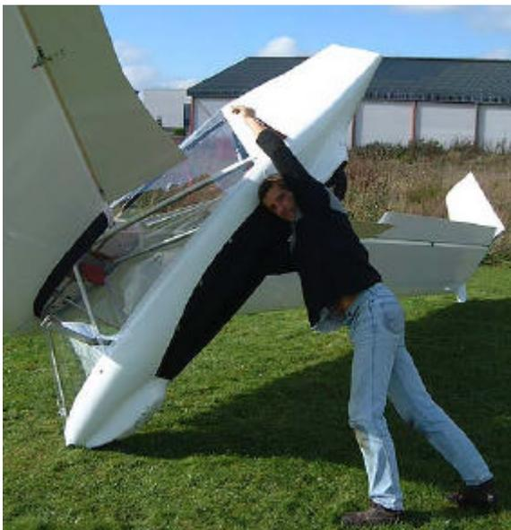
3. Put the **right hand** inside the trap doors, pass **over** the hammock and grab the right longitudinal tube.
