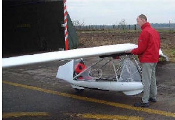
1. On **nice ground**, one can roll it. Put the flaps at 0° and push backwards by pushing on the nose. Slightly lifting the nose with flat hands on the under surface.
