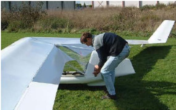
1. Make sure the hammock is in slack position. With the aid of the little strap found on the left hand side of the tail cone, grab this handle by pulling the lower strand. *If you pull it out holding top and bottom strand it may not retract automatically.*
