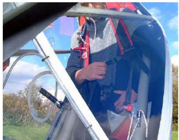
8. Clip together the little clips between the shoulder straps and then adjust it. *The glider should be well balanced and requires very little effort.*
