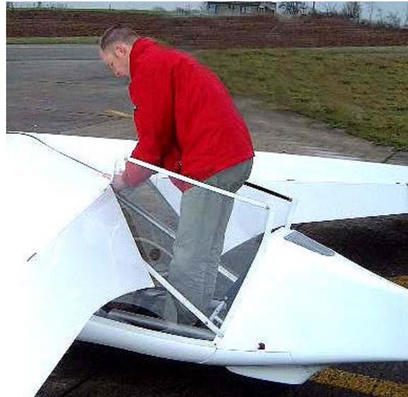
2. Stand up on the Hammock using the trailing edge to balance. **Do not lean on the fairing.**
